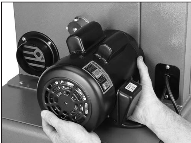
Figure 13. Installing motor (outside view).
